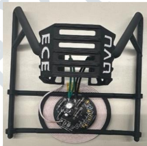
Fig. 9. Construction of the landing gear using 3D printer.
