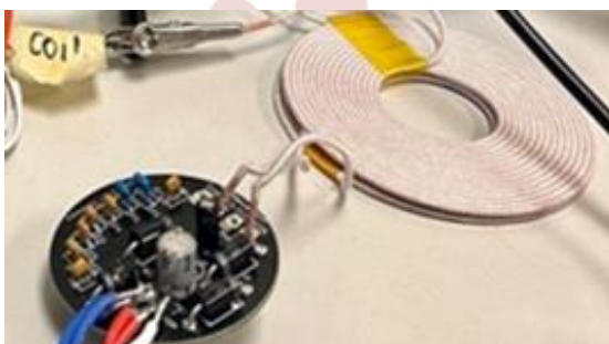
Fig. 8d. Constructed prototype of the receiver.
